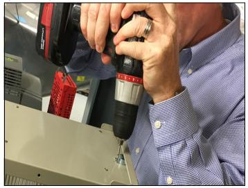
6. Replace the door latch, and insert the supplied screws in the existing holes.
