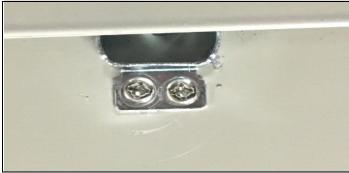
7. Install the supplied nuts to the back of the screws and tighten with a Phillips head screw driver and hex key.
