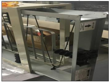
5. Use a 1/8-inch drill bit to drill out the door latch rivets.
