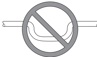
Fig. 21 - Insufficient Condensate Trap
