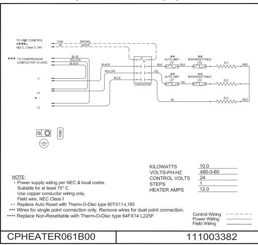
Fig. 22 – CPHEATER061B00 Wiring Diagram
