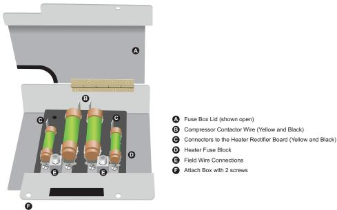
Fig. 11 – Schematic Location for Non-Fused Heater
