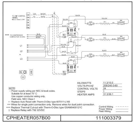
Fig. 20 - CPHEATER058B00 Wiring Diagram
