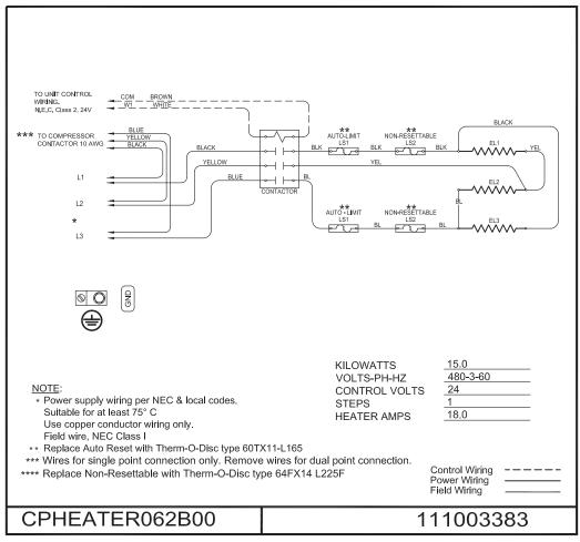
Fig. 24 - CPHEATER063B00 Wiring Diagram
