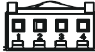
Fig. 20 – Sensor Wire Harness Pin Layout
