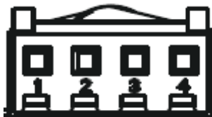
Fig. 20 – Sensor Wire Harness Pin Layout
