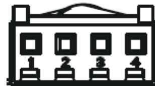
Fig. 13 – Sensor Wire Harness Pin Layout
