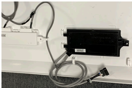
Fig. 23 — Front Panel with New Display Board and Adapter Board
