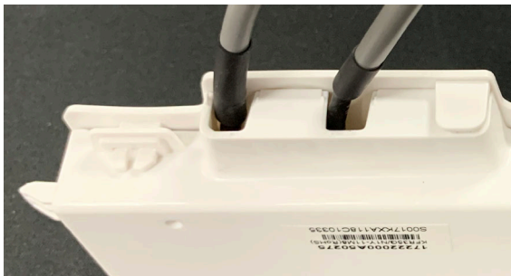
Fig. 15 — CN101 Connection to the Adapter Board
