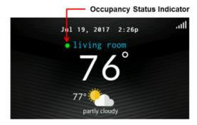
The Occupancy Sensing feature can be enabled or disabled by the installer.
