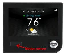
The on-board PIR motion sensor is placed on the bottom left corner of the Connex™ Control. It is able to detect motion at least 25 feet directly in front of the sensor, and within 135° cone perpendicular to the wall. The motion detection pattern is shown as below.
