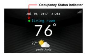
The Occupancy Sensing feature can be enabled or disabled under the 'sensors' icon.
