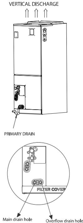
**Fig. 30 —Vertical Discharge**
