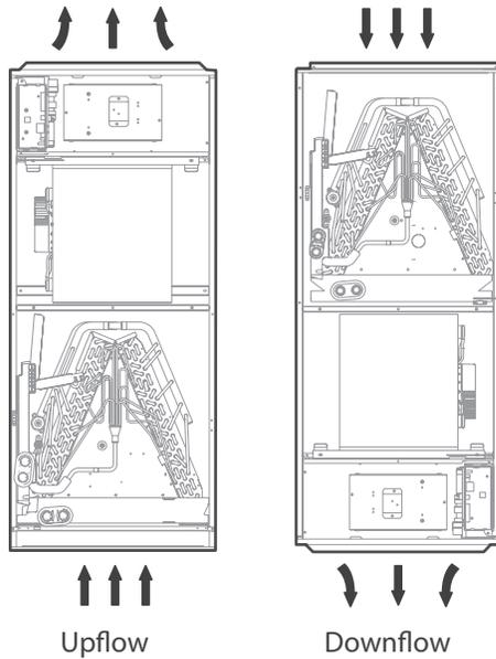
**Fig. 11 — Vertical Airflow**
