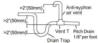
**Fig. 31 — Vertical Discharge**
