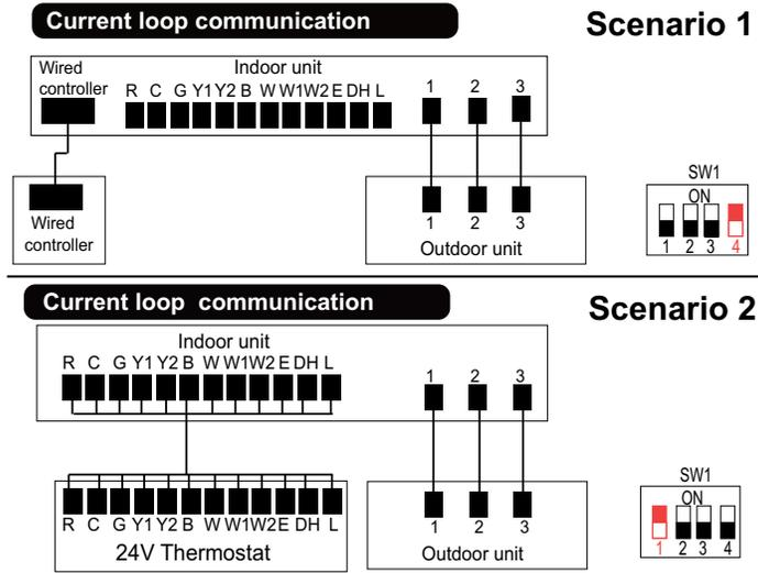
Fig. 52 —Connection Methods for 18K-36K Residential Units
