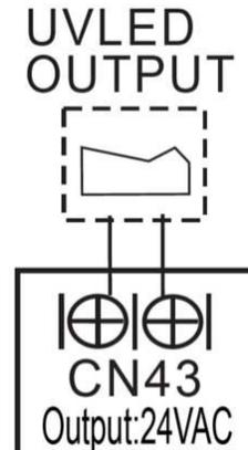
**Fig. 62 —UV LED Terminal Port CN43**
