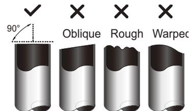
Fig. 33 —Pipe Cutting
