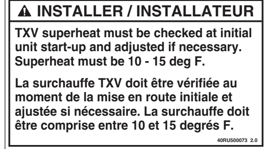
Fig. 30 — TXV Adjustment Label
