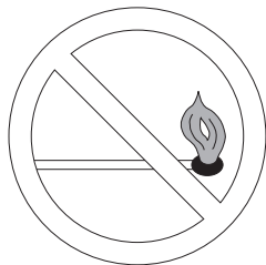
Fig. 2 – Do Not Light Burner with Match
