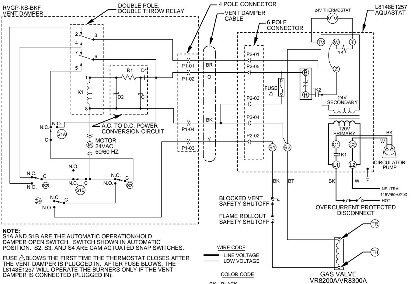
**NOTE:** If any of the original wire as supplied with this appliance must be replaced, it must be replaced with type 105°C thermoplastic wire or its equivalent.
