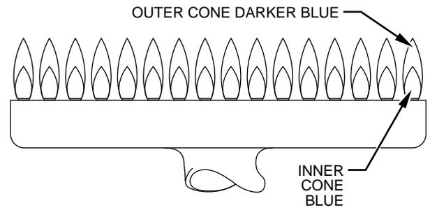
Fig. 17—Main Burner Flame
