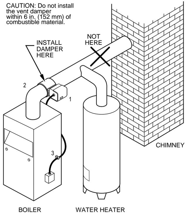
1. Install the vent damper to service only the single appliance for which it is intended. If improperly installed, a hazardous condition, such as an explosion or carbon monoxide poisoning, could result.
