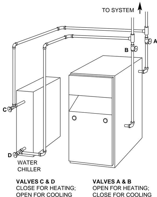
**Fig. 4—Chilled Water Piping**
