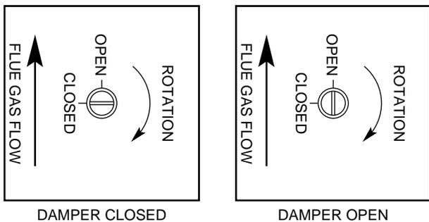
**Fig. 7—Effikal Vent Damper Position Indicator** A95147
