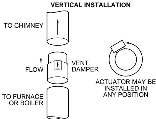
**Fig. 6—Horizontal and Vertical Vent Damper Installation** A95145
