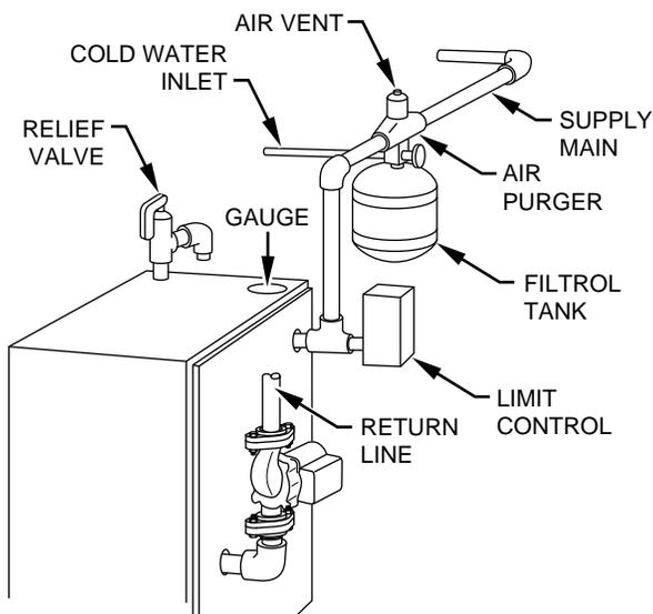
**Fig. 3—Typical Hot Water Piping**
