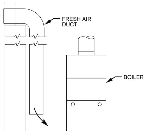
**Fig. 2—Fresh Air Duct for Tightly Sealed House**
