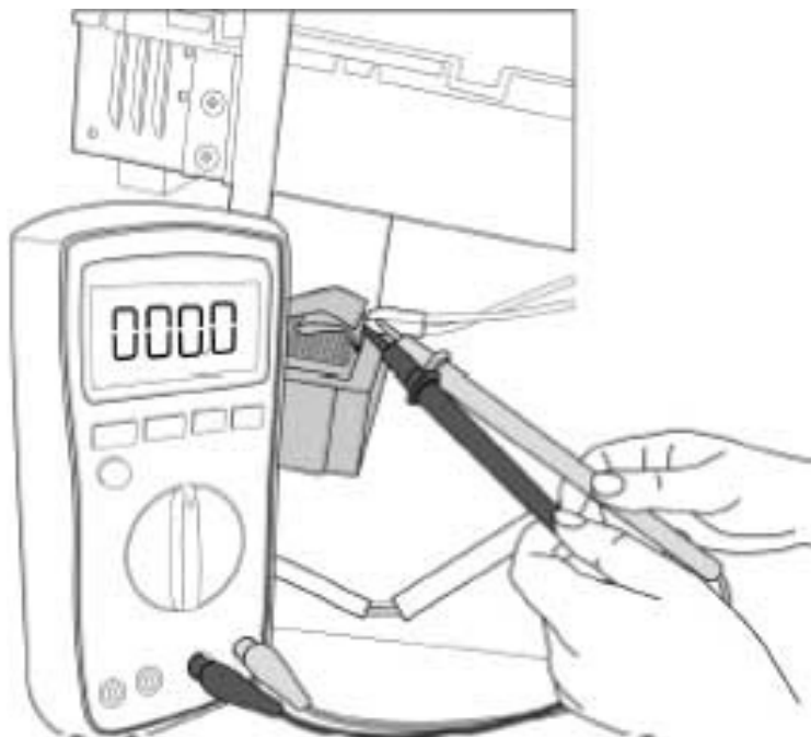
Fig. 43 —Test Resistance of Reactor with Multimeter
