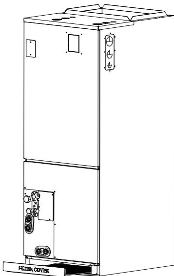
**Fig. 27 —Reinstall Filter and Cover Plate**
