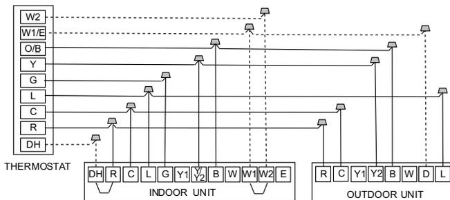
**Fig. 66 —Wiring for 3H and 1C Thermostat**
