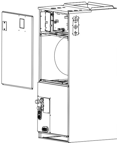
**Fig. 16 —Remove Upper Cover Assembly**
