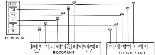
**Fig. 69 —Wiring for 2H and 2C Thermostat**
