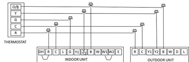
**Fig. 71 —Wiring for 1H and 1C Thermostat**
