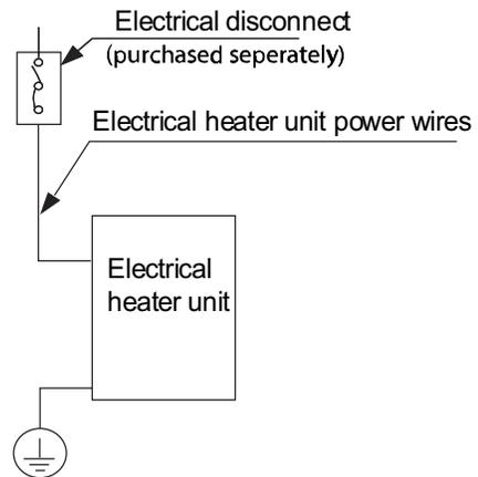
**Fig. 48 — Electrical Disconnect**
