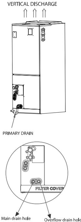
**Fig. 29 —Vertical Discharge**
