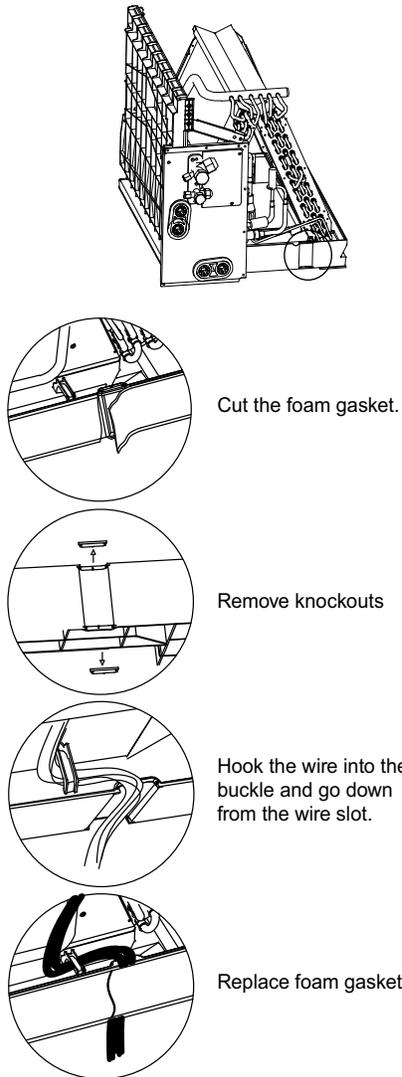
**Fig. 23 —Reinstall Sensor Plugs and Electronic Expansion Valve**
