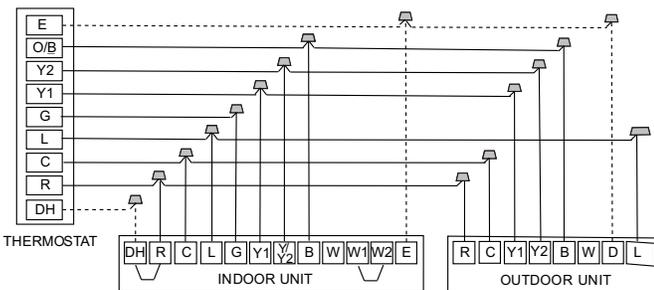
**Fig. 67 —Wiring for 3H and 2C Thermostat**
