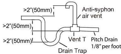
**Fig. 30 — Vertical Discharge**
