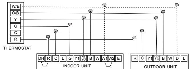
**Fig. 70 —Wiring for 2H and 1C Thermostat**
