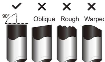
**Fig. 32 —Pipe Cutting**
