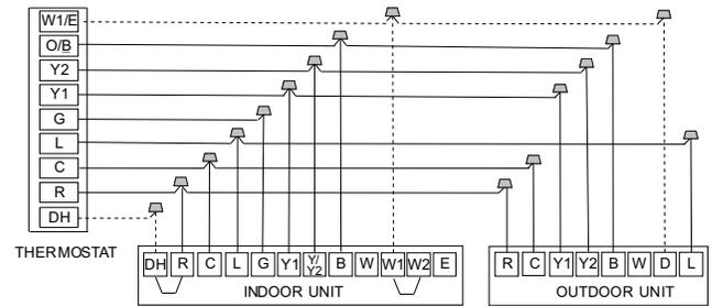
**Fig. 68 —Wiring for 3H and 2C Thermostat**
