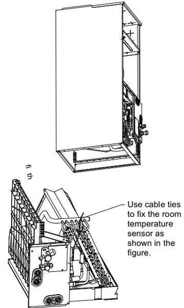
**Fig. 24 —Assembled Evaporator**
