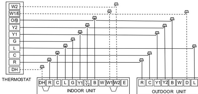
**Fig. 65 —Wiring for 4H and 2C Thermostat**
