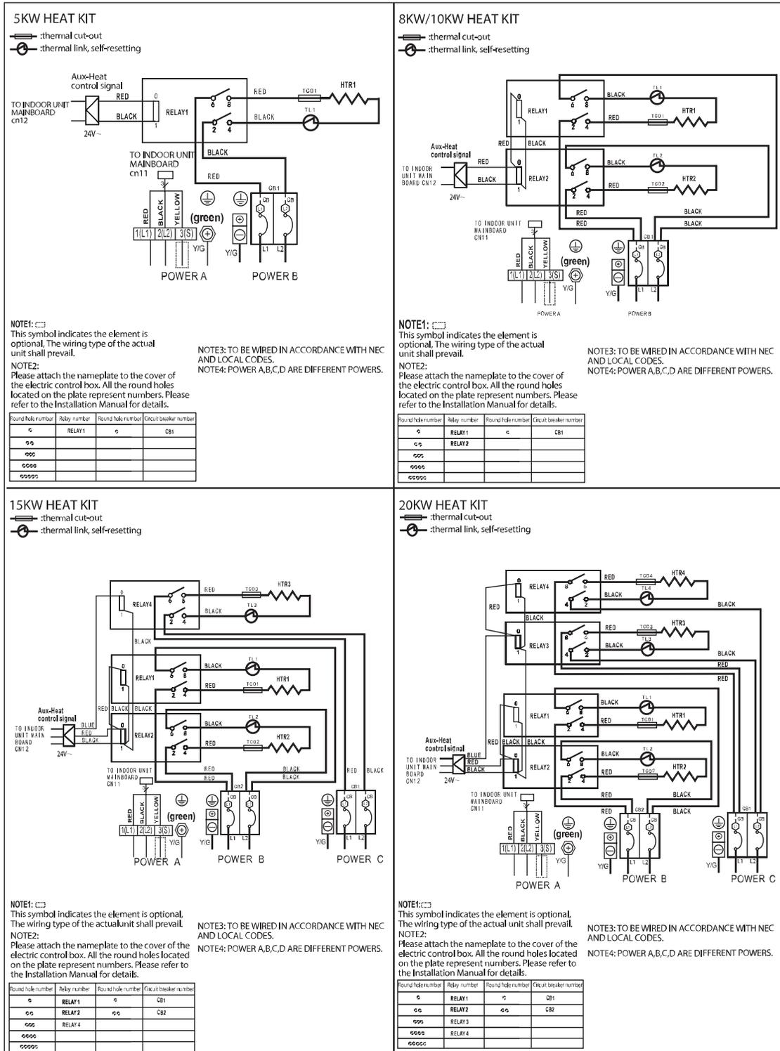
Fig. 63 — Electric Auxiliary Heating Wiring Diagram
