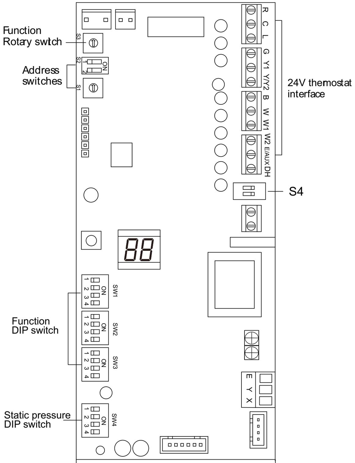
Fig. 54 — DIP Switches
