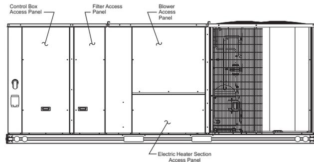
**Fig. 33 - Typical Access Panel Location**
