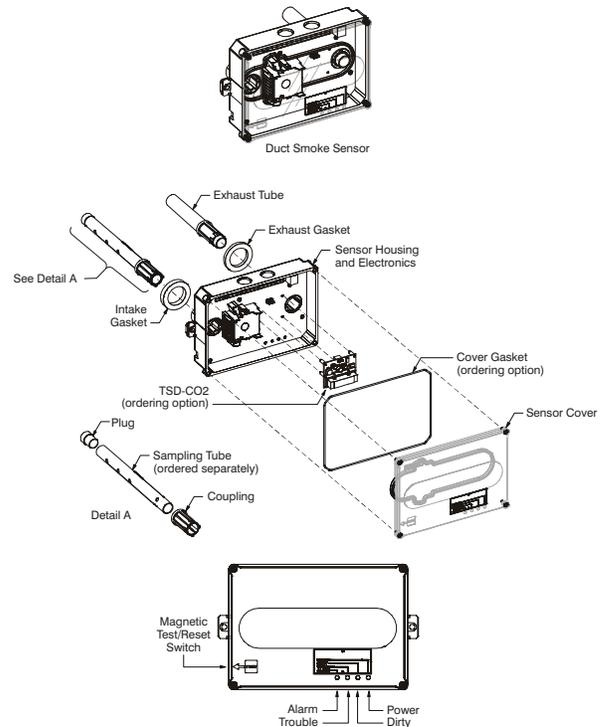
**Fig. 40 - Smoke Detector Sensor**
