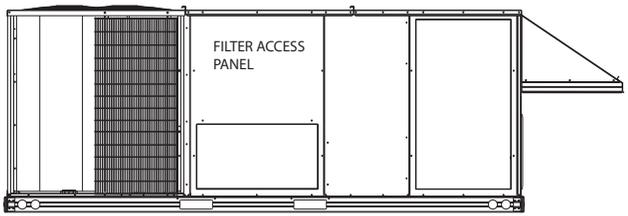
Fig. 2 - Typical Access Panel Locations (Rear)
