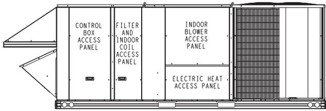
Fig. 1 - Typical Access Panel Location (Front)
