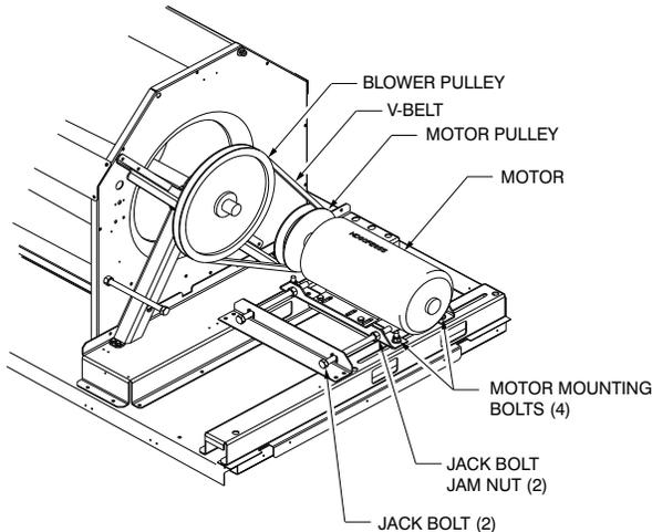
**Fig. 6 - Replacing the V-Belt**
