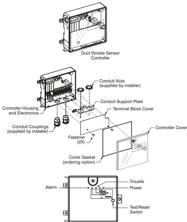
**Fig. 39 - Controller Assembly**
