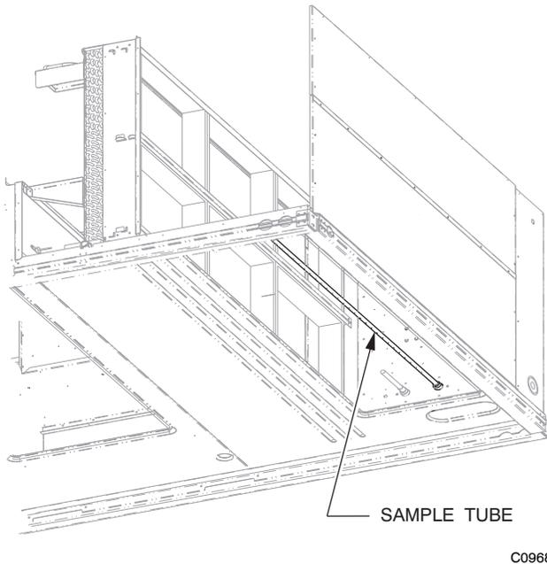
**Fig. 44 - Return Air Detector Shipping Position**
