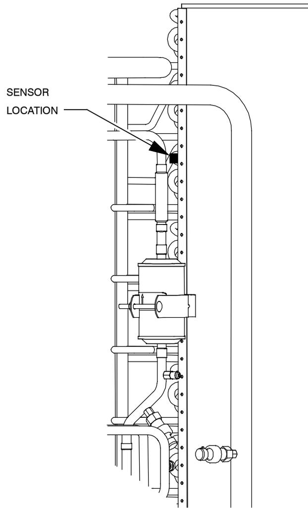
**Fig. 59 - 50TCQD17 and 50TCQD24 Motormaster Sensor Location**
