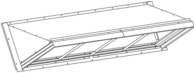
**Fig. 3 - Screens Installed on Outdoor-Air Hood**
