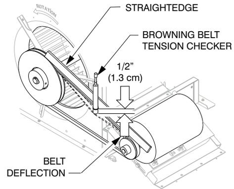
**Fig. 5 - Checking Blower Motor Belt Tension**
