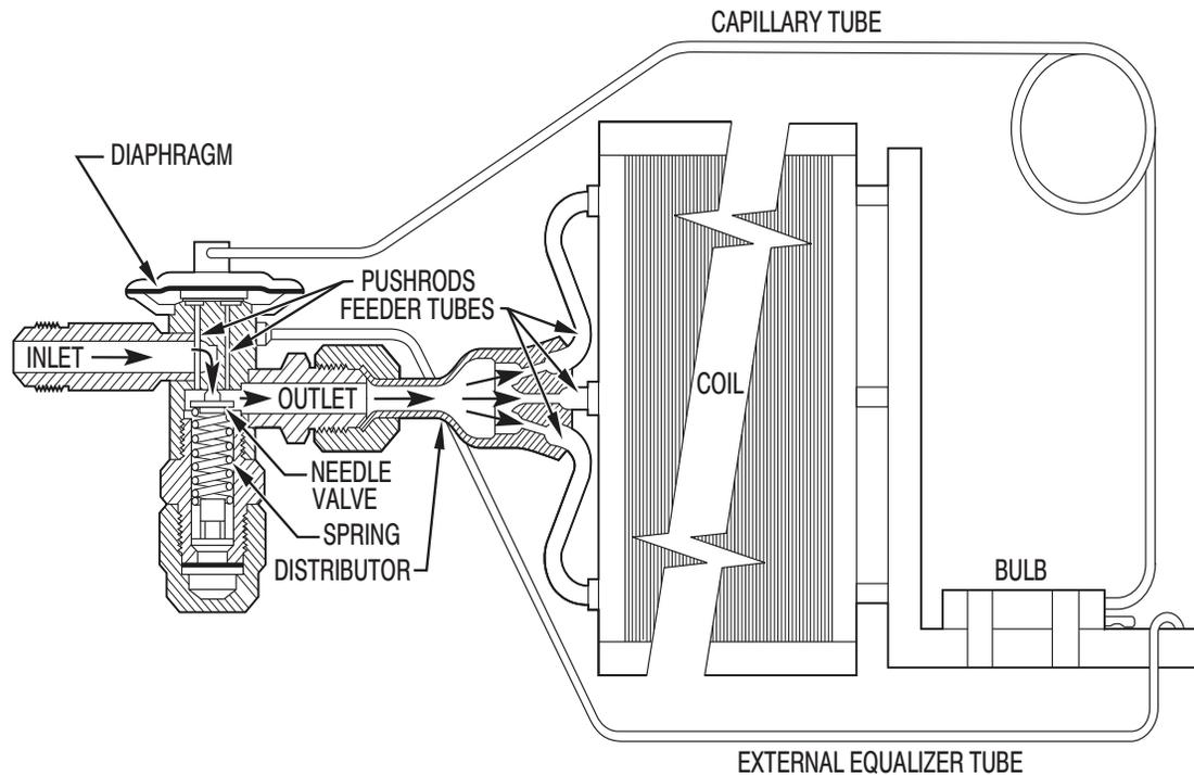
**Fig. 19 - Thermostatic Expansion Valve (TXV) Operation**
