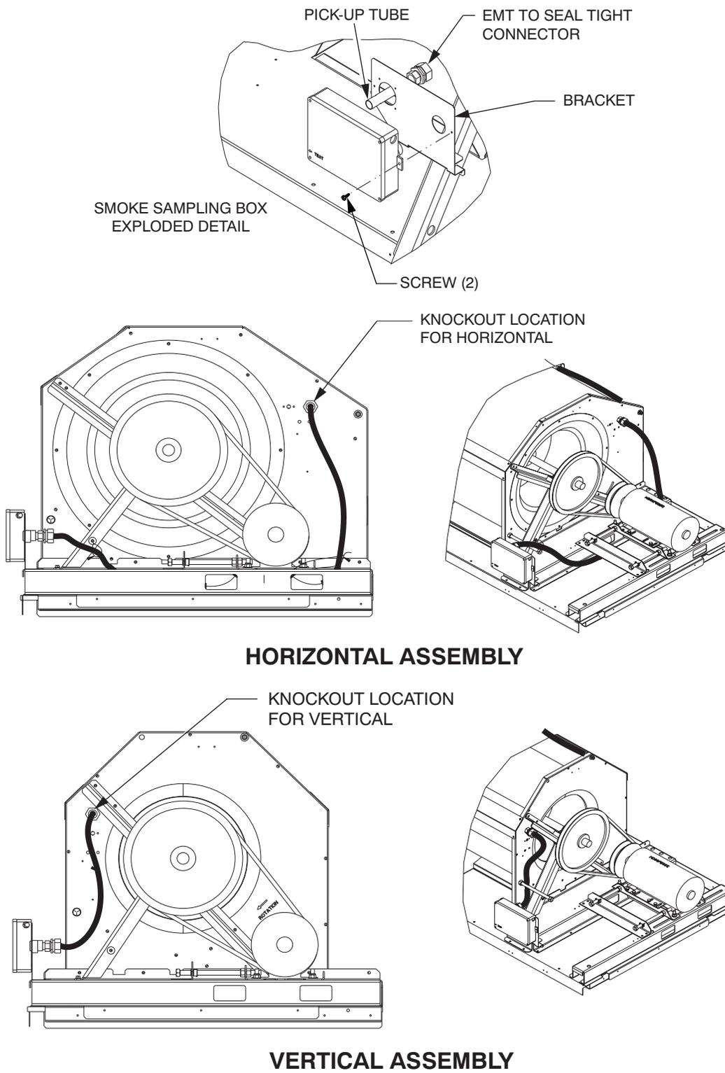
**Fig. 45 - Supply Air Smoke Detector Sensor Location**
