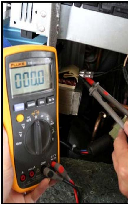
**Fig. 24 – Test the Reactor Resistance**
