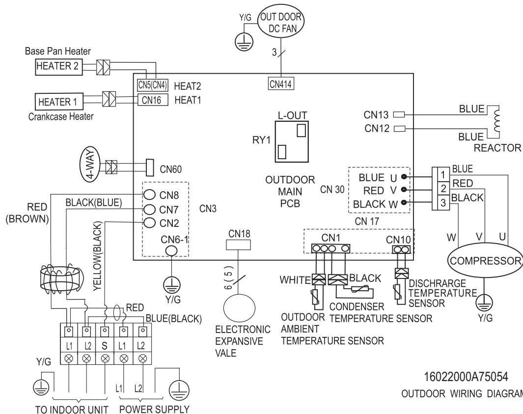
**Fig. 10 — Wiring Diagram - Sizes 09K, 12K, 18K (208-230V)**
