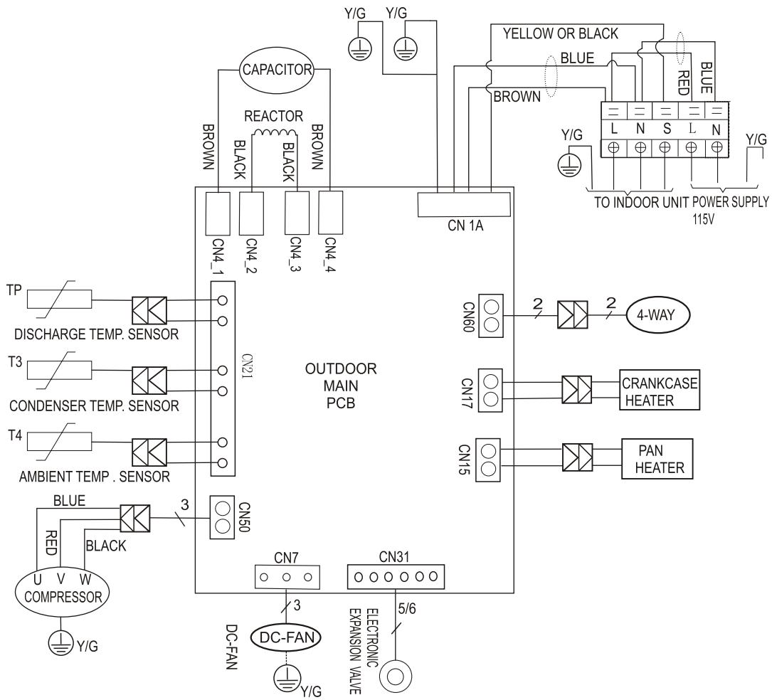
Fig. 9 — Wiring Diagram Size 12K (115V)
