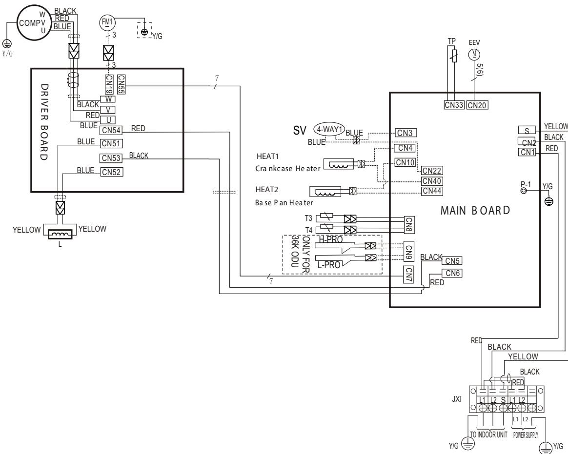
Fig. 11 — Wiring Diagram Sizes 24K - 36K
