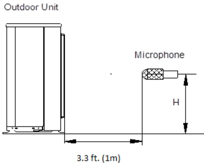
Fig. 8 — Outdoor Unit Sound Pressure Test
