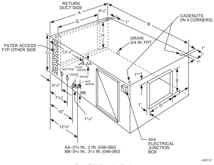
Fig. 1—FG3A Dimensional Drawing
