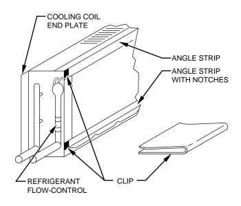
Fig. 4—Installing Angle Strips
