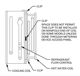
Fig. 5—Securing Hot-Water Coil
