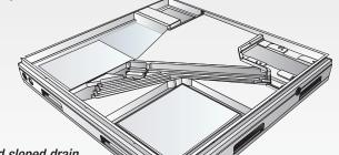
The integrated sloped drain pan design minimizes the amount of condensate that remains in the indoor air cavity, reducing the opportunity for mold, mildew and odors to form.
