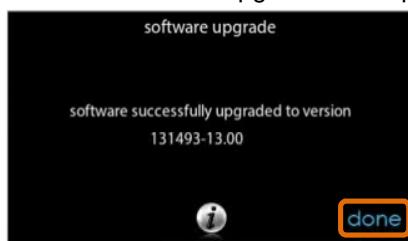
13. The Infinity® Touch control will perform a restart after the **DONE** button is pressed. There will be a longer than normal delay for the wall control to restart since part of the process at this time is the completion of the new software installation. Once the Infinity® Touch control has successfully restarted, the USB device may be removed.
