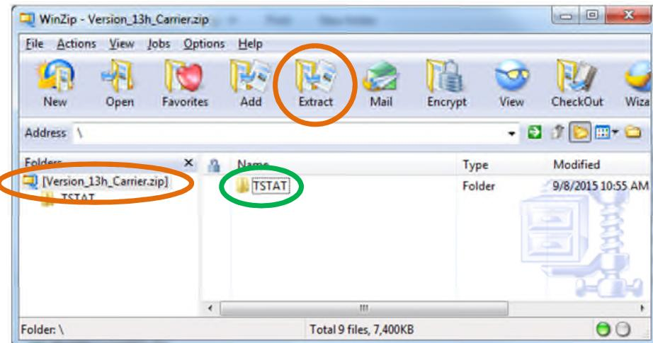
6. Choose the USB memory device as the location to extract the folder from the zip file. This will over-write the existing TSTAT folder any files contained within it. Click Extract.
