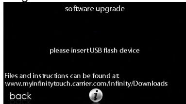
11. If the .hex file is stored properly on the USB drive, this screen will appear. If the screen says, "Please insert USB Device", remove the USB drive and re-insert. If it still does not show the screen, below, go back to Step 5. Verify that the "update software version" reads 131493-13; note that there may be a later sub-version shown after the "13." Press **YES** to continue with the software upgrade. The upload and installation will take several minutes.
