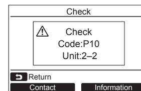
While the check information screen appears: Push the [Contact] button [F1] to display the contact number for service. Push the [Information] button [F2] to display the model name and serial number of the unit.
