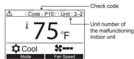
When an error has occurred in the air conditioner, the check code and the unit number of the indoor unit appear on the display of the remote control.
