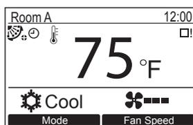
Clean the air filter when “
