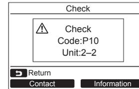
While the check information screen appears: Push the " Contact " [ F1 ] button to display the contact number for service. Push the " Information " [ F2 ] button to display the model name and serial number of the unit.
