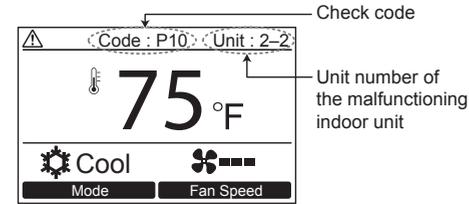
When an error has occurred in the air conditioner, the check code and the unit number of the indoor unit appear on the display of the remote control.
