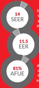
SEER (Seasonal Energy Efficiency Ratio) is an average measure of how efficiently your air conditioner uses electricity to provide cooling.
