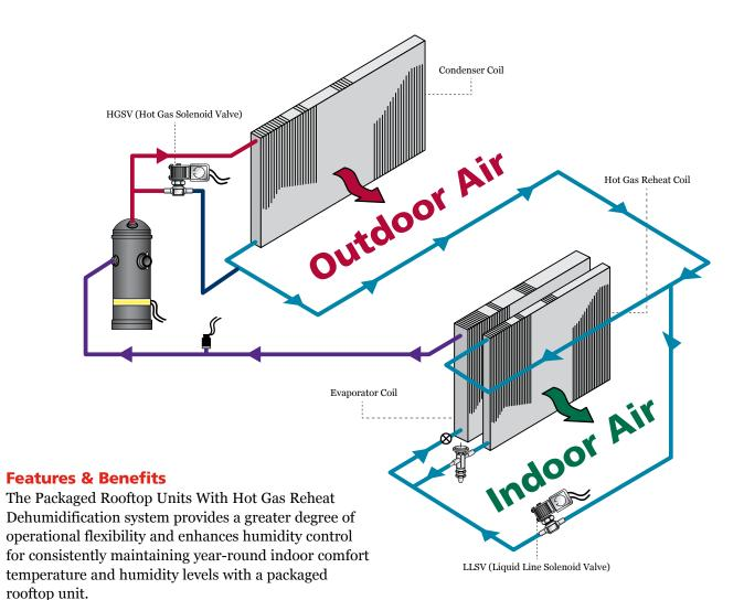
**Superior Humidity Control** – Using compressors for active dehumidification, the system can boost the latent capacity of the standard rooftop unit by up to 40% in the sub-cooling mode and still allow the capability for dehumidification without a call for cooling, when required by the space.
