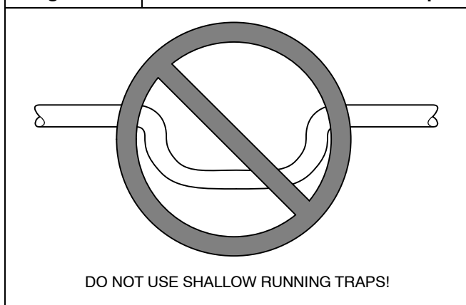
Figure 15 Insufficient Condensate Trap
