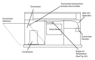
Fig. 8 - Routing Harness Extension and Mounting SAT Sensor
