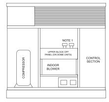
NOTE 1: Field provided relays can be mounted on top of upper block off panel, if applicable Location for heat pump relay package number CPRLYKIT001A00.
