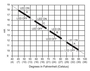
Fig. 15 - Outdoor Air Temperature Changeover Set Points
