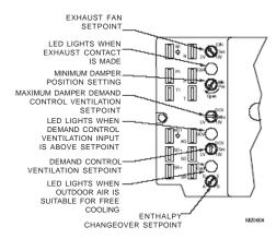
Fig. 14 - Economizer Controller Potentiometer and LED Locations
