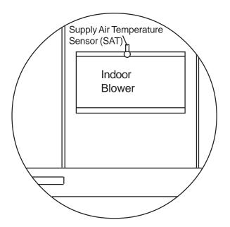
Fig. 9 - SAT Location for Units Wihout Block Off Panel
