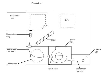
Fig. 10 - Routing Harness (Top View)
