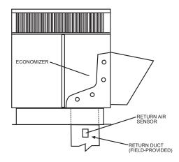
Fig. 16 - Return Air Temperature or Enthalpy Sensor Mounting Location
