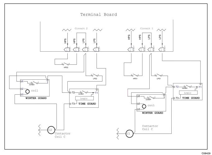
Fig. 9 - Wiring Diagram, Time Guard II Device with Winterguard for 3 to 12-1/2 Ton Units (1 and 2 Compressor Systems) with R-410A Refrigerant
