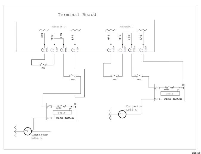
Fig. 8 - Wiring Diagram, Time Guard II Device for 3 to 12-1/2 Ton Units (1 and 2 Compressor Systems) with R-410A Refrigerant
