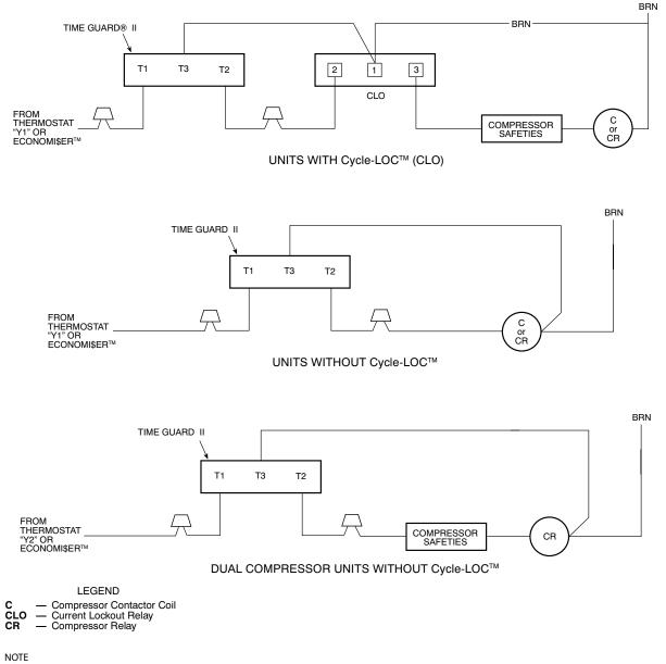
Fig. 6 - Wiring Connections, 3 to 12-1/2 Ton Small Rooftop Units with R-22 Refrigerant
