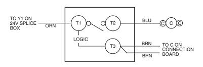
Fig. 11 - Wire Connections, 6 to 10 Ton Condensing Units
