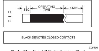
Fig. 2 - Time Guard II Device Sequence Chart
