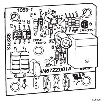
Fig. 1 - Solid-State Time Guard II Device
