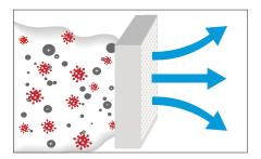
Kill Captured airborne microbes remain on the pleated filter instead of recirculating back into the home and are subjected to an intense electric field. There, 99% of select viruses and bacteria are inactivated.<sup>1</sup>
