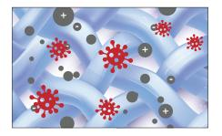
**Capture** The ionized particles are pulled toward an oppositely charged, pleated MERV 15 rated filter and captured at an extremely high rate, similar to how a magnet attracts metal shavings.<sup>7</sup>
