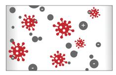
**Charge** The purifier creates a "cloud" of electrically charged ions that attach themselves to airborne dust, pollen, viruses, germs and other particles as they pass through.
