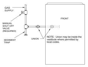
Fig. 31 – Typical Gas Pipe Arrangement
