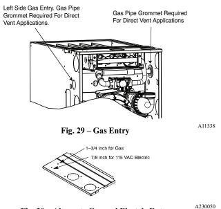
Fig. 30 – Alternate Gas and Electric Entry
