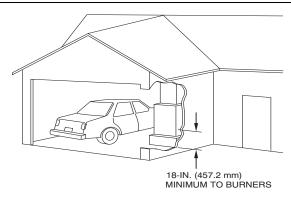
Fig. 5 – Installation in a Garage
