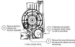
Unconverted Factory Configuration As Viewed in the Horizontal Right Orientation
