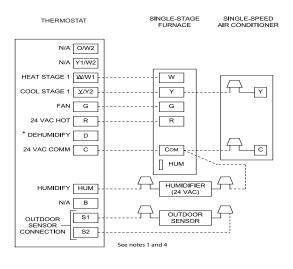
Single-Stage Furnace with Single-Speed Air Conditioner
