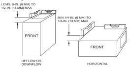
Fig. 19 - Furnace Pitch Requirements
