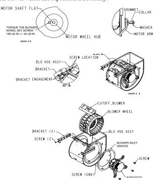
Fig. 62 - Blower Assembly on 0401410 and 0401412
