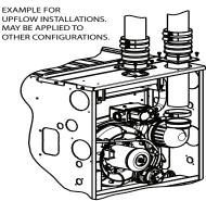
Fig. 43 – Sample Inlet Air Pipe Connection for Polypropylene Venting Systems
