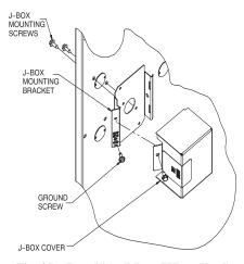
Fig. 35 – Installing J-Box (When Used)
