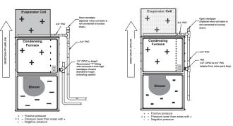
Fig. 12 - Example of Field Drain Attachment
