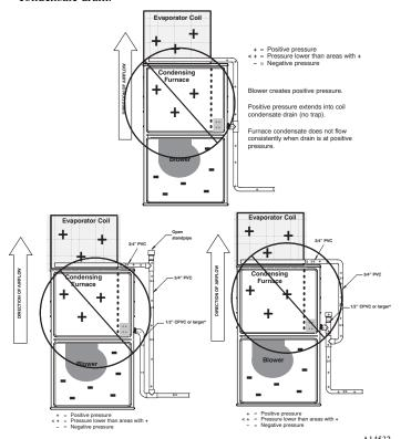
$\textbf{Fig. 13-Example of Field Drain Attachment (Not Allowed)}^{\text{A14532}}$
