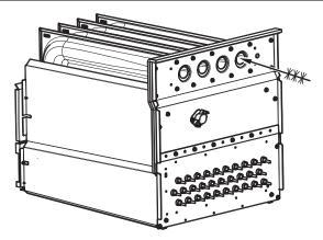
Fig. 67 – Cleaning Heat Exchanger Cell
