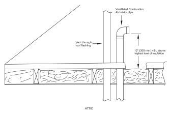
Fig. 46 – Vent Terminations for Ventilated Combustion Air
