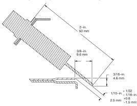
Fig. 66 – Igniter Position - Side View
