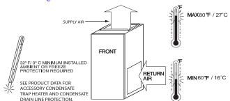
Fig. 3 – Freeze Protection and Return Air Temperature
