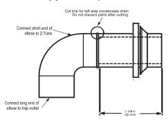
Fig. 17 - Modify Rubber Drain Elbow
