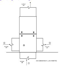
Fig. 21 – Upflow Return Air Configurations and Restrictions  $^{\rm A11036}$
