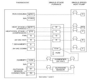
Single-Stage Furnace with Single-Speed Heat Pump
