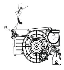
Fig. 58 – Priming Condensate Trap
