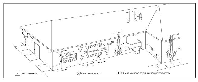
Fig. 41 – Direct Vent Termination Clearance
