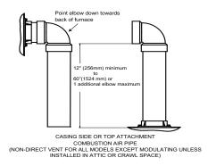
Fig. 44 – Combustion Air Pipe Attachment
