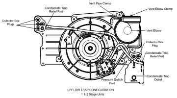
Fig. 8 – Upflow Trap Configuration
