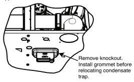
Fig. 18 – Horizontal Drain Trap Grommet
