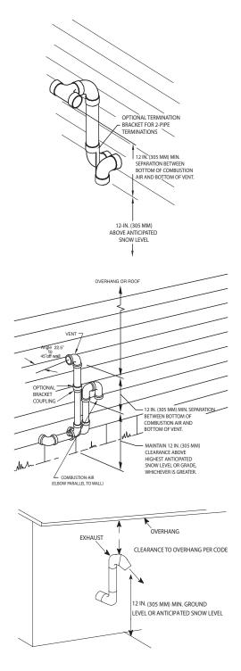
Fig. 48 – Alberta and Saskatchewan Vent Termination Algorithm Size the Vent and Combustion Air Pipes General
