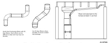
Fig. 51 - Near Furnace Vent Connections
