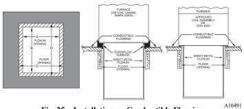
Fig. 25 – Installation on Combustible Flooring
