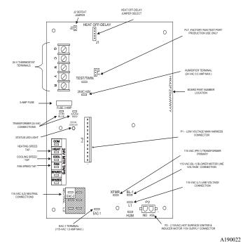
Fig. 37 - Example of Single Stage Furnace Control
