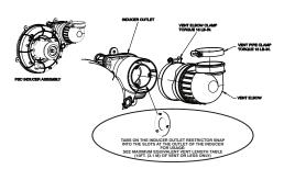
Fig. 52 – Inducer Vent Elbow
