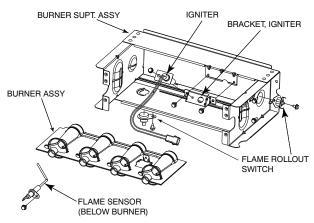
Fig. 64 – Burner Assembly
