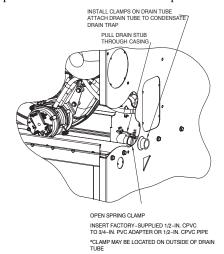
Fig. 14 - Formed Rubber Drain Grommet
