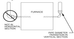
Fig. 49 – Combustion Air and Vent Pipe Diameter Transition A93034 Location and Elbow Configuration
