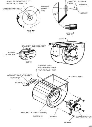
Fig. 63 – Blower Assembly on 1002122
