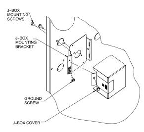
Fig. 33 – Installing J-Box (When Used)
