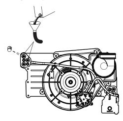
Fig. 60 – Priming Condensate Trap
