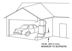
Fig. 5 – Installation in a Garage
