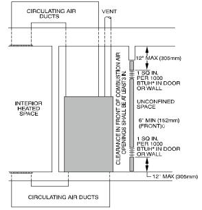
Minimum opening size is 100 sq in. (64516 sq. mm) with minimum dimensions of 3-in. (76mm)
