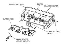
Fig. 66 - Burner Assembly
