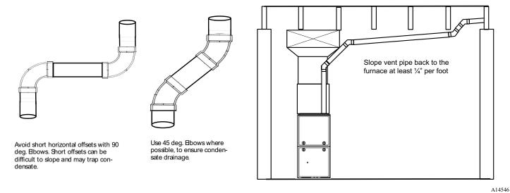
Fig. 52 - Near Furnace Vent Connections
