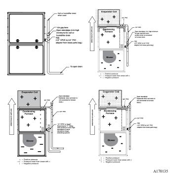
Fig. 12 – Example of Field Drain Attachment
