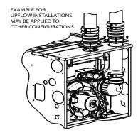
Fig. 40 – Sample Inlet Air Pipe Connection for Polypropylene
