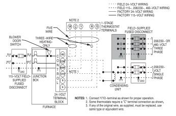
Fig. 36 – Typical Two-Stage Field Wiring Diagram
