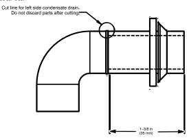
Fig. 17 - Modify Rubber Drain Elbow
