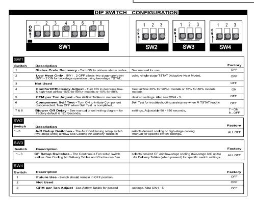
Fig. 59 – Furnace Setup Switches and Description
