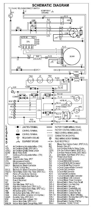
Fig. 71 - Wiring Diagram
