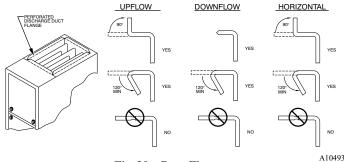
Fig. 20 - Duct Flanges
