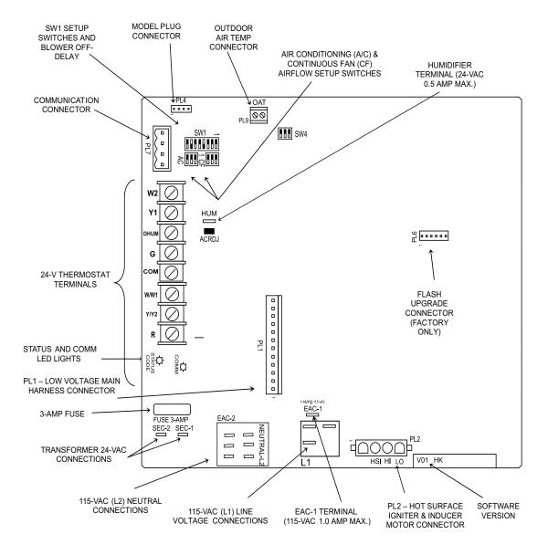
Fig. 38 – Example of Variable Speed Furnace Control
