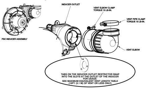
Fig. 53 – Inducer Vent Elbow
