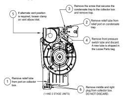
Unconverted Factory Trap Configuration
