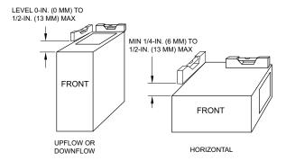
Fig. 19 – Furnace Pitch Requirements
