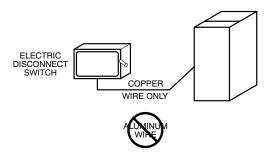
Fig. 32 – Field-Supplied External Electrical Box on Furnace Casing
