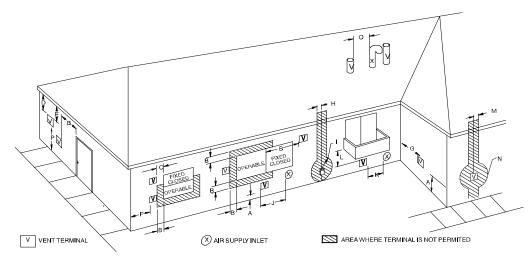
Fig. 45 – Direct Vent Termination Clearance
