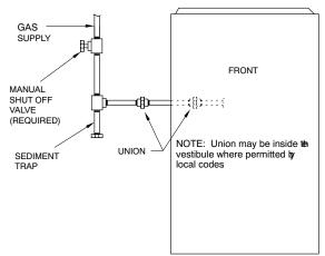
Fig. 31 – Typical Gas Pipe Arrangement
