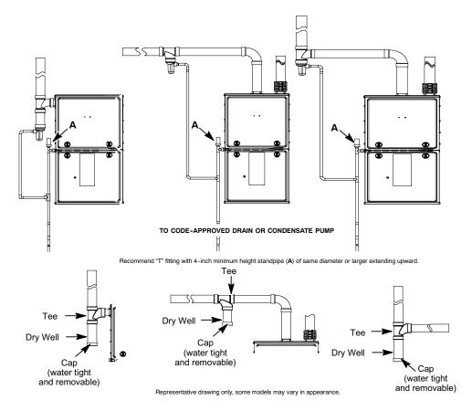
Fig. 50 - Recommended Combustion Air Inlet Moisture Trap
