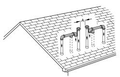
Fig. 44 – Pipe Vent and Combustion
