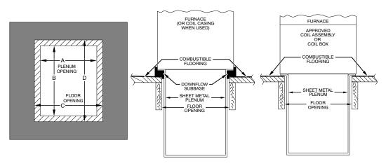
Fig. 25 - Installation on Combustible Flooring
