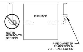
Fig. 49 – Combustion Air and Vent Pipe Diameter Transition
