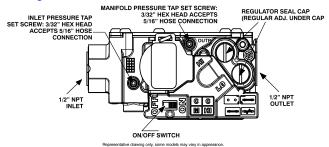
Fig. 62 – Gas Valve with Tower Pressure Ports
