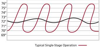
Low-Stage Operation of a Two-Stage Unit – \* Performance may vary depending on thermostat used.
