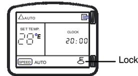
Use this function to lock the settings on the remote control and to prevent the settings being changed.
