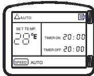
Use both functions to program the unit to turn on and shut off at specified times.
