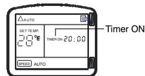
This function will allow the unit to start automatically after a set number of hours. The TIMER ON can be set while the unit is on or off.
