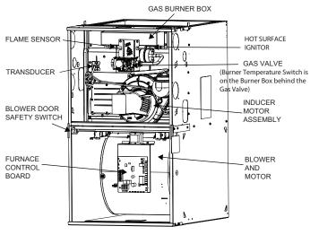
Fig. 1 – Furnace Components
