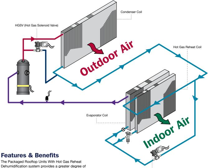
The Tempstar® tradition of delivering reliable, economical comfort that customers can trust continues with our Packaged Rooftop Units With Hot Gas Reheat Dehumidification system. As a direct result of more cost-effective systems, these packaged rooftop units are currently being implemented in expanded applications, many of which require the highest degree of indoor comfort and humidity control.
