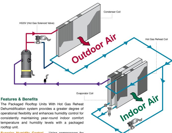
operational flexibility and enhances humidity control for consistently maintaining year-round indoor comfort temperature and humidity levels with a packaged rooftop unit.
