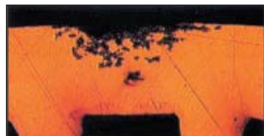
Fig. 2 Formicary Corrosion Tunneling
