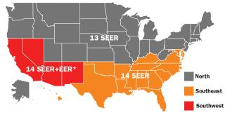
On January 1, 2015, a new set of minimum efficiency standards took effect. Under the new standards, there are different efficiency minimums for air conditioners in each of three regions—North, Southeast and Southwest. The national minimum efficiency standard for heat pumps is 14 SEER/8.2 HSPF.
