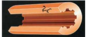
3-D representation of corrosion through tube
