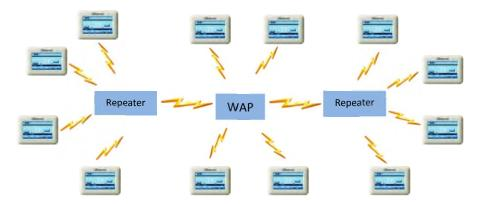
This information may also be useful if you are having trouble with signal strength due to obstructions between the router or WAP and a wall control. A repeater may be placed in a way that allows the wireless signal to be directed around an obstruction. See the figure, below.
