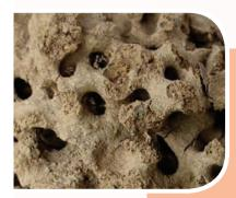
Formicary corrosion, sometimes called "ant's nest" corrosion, appears as multiple tiny pinhole leaks at the surface of a copper tube that are not visible to the human eye. These tiny leaks break down the strength of the copper tubing and can ultimately cause coil failures.
