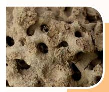
Formicary corrosion, sometimes called "ant's nest" corrosion, appears as multiple tiny pinhole leaks at the surface of a copper tube that are not visible to the human eye. These tiny leaks break down the strength of the copper tubing and can ultimately cause coil failures.
