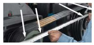
Straightedge must make contact at 4 distinct points along the outside perimeter of both pulleys
