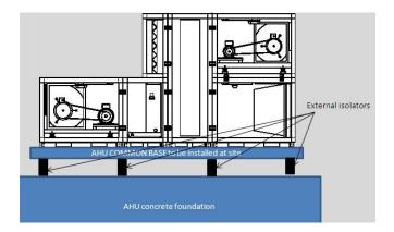
In case of multi section unit It is highly recommended to install common (single channel base through the AHU) base channel underneath the AHU. Rubber pads/ isolators will be installed underneath this single channel base.
