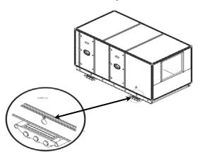
For horizontal movement pallet lifters or transport skids can be placed under the installation frame or under the lifting bars. It is important that these support the lifting points. At no time should the cross beams at the ends of the unit sections be used for jacking or tracking the AHU. FOR HORIZONTAL TRANSPORT ALWAYS PROVIDE SUPPORT UNDER THE LIFTING POINTS.
