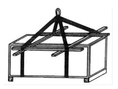
2) To the lifting bars. (Lifting bars are not supplied by factory )
