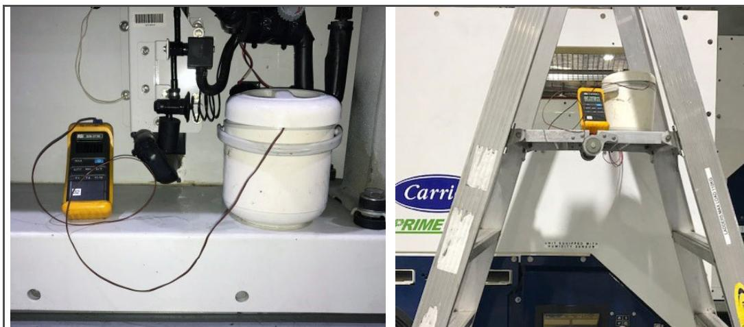
7. Once temperature stability is ensured, submerge the sensors in the ice water slurry. Make certain that the sensors do not contact the container sides or bottom, or each other. Continuously stir the slurry mixture during calibration.
