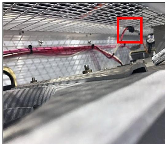
4. Cut all the wire ties that are securing the sensors to the harness and remove sensor.
