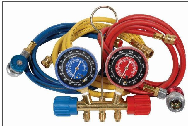
The gauge set layout with hoses and couplings is shown in **Figure 7.2**. The gauge set connects to the service connections on the refrigeration unit using the blue and red hoses. Service connections are described in **Section 7.1.3**. The yellow hose is a utility connection that can be connected to a refrigerant cylinder or vacuum pump.
