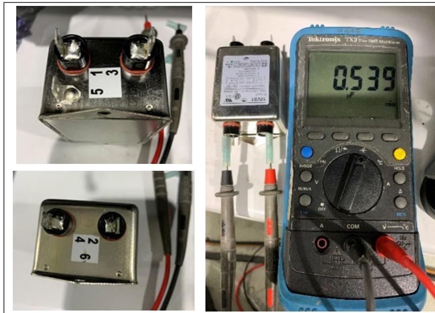
5. Each individual pin can also be verified between the ground pin #5 and 1, 2, 3, 4. Testing each individual pin to the ground pin should read a capacitance of  $0.011 \mu\text{F} \pm 10\%$ . Note that meter to left reading in nF but passing value 0.01052  $\mu\text{F}$ .
