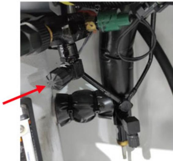
4. Apply lubricant (46-00058-00) on the o-ring of the high side charge port (40-00812-01). Replace the current charge port with the new charge port. Use 2 wrenches and tighten to 65 lbf-in.
