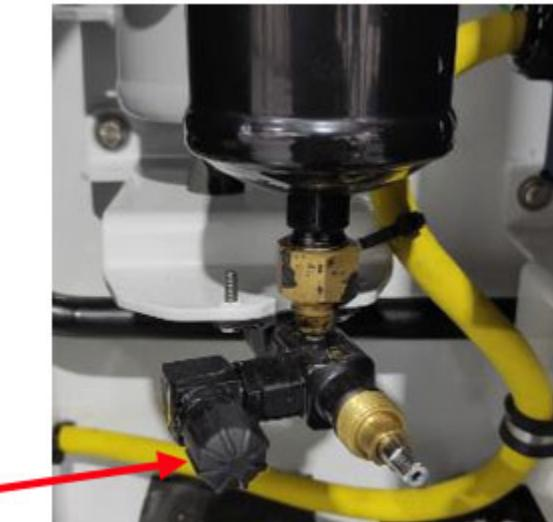
2. Apply lubricant (46-00058-00) on the o-ring of the high side charge port (40-00812-01). Replace the current charge port with the new charge port. Use 2 wrenches and tighten to 65 lbf-in.
