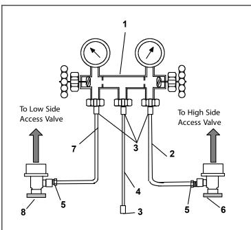
Figure 7.2 R-134a Manifold Gauge/Hose Set
