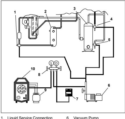
Figure 7.4 Refrigeration System Service Connections
