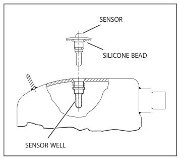
Figure 7.19 Compressor Discharge Temperature Sensor
