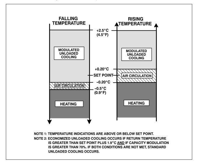
Figure 4.5 Controller Operation - Perishable Mode
