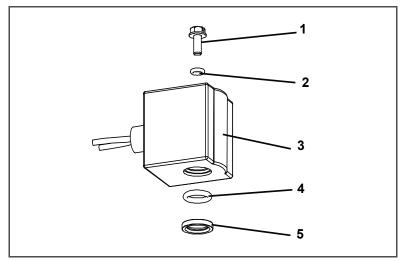
Figure 7.11 Coil View of Economizer Solenoid Valve (ESV)
