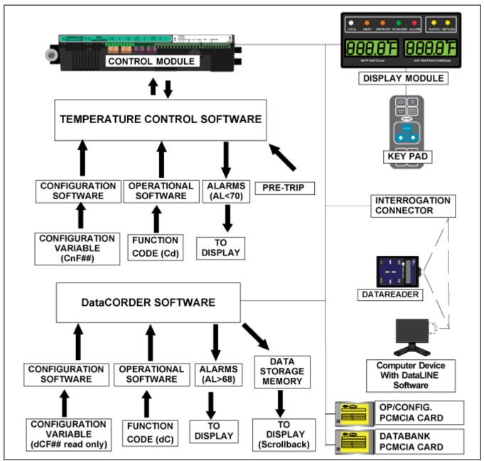
Figure 4.1 Temperature Control System
