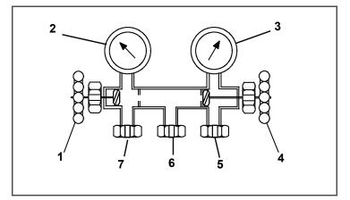
Figure 7.1 Manifold Gauge Set
