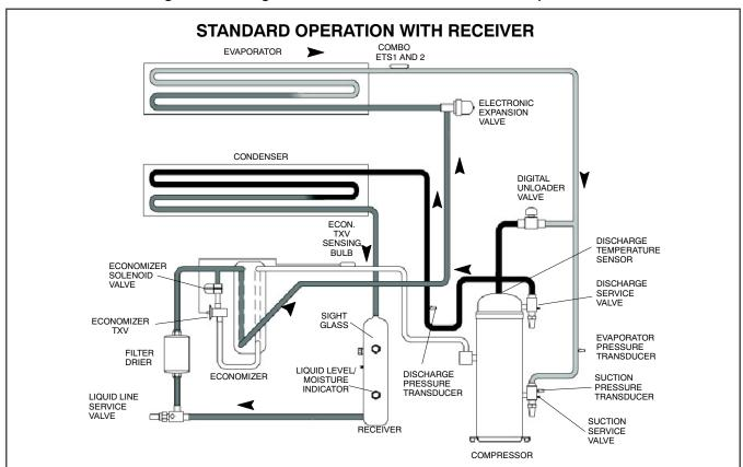
Figure 3.6 Refrigeration Circuit Schematic - Standard Operation
