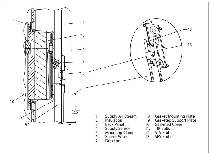
Figure 7.17 Return Sensor Positioning
