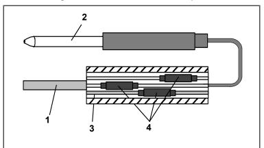
Figure 7.15 Sensor and Cable Splice
