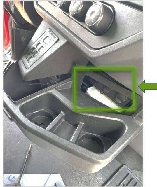
DO NOT replace the center console until after checking the Gateway device status
