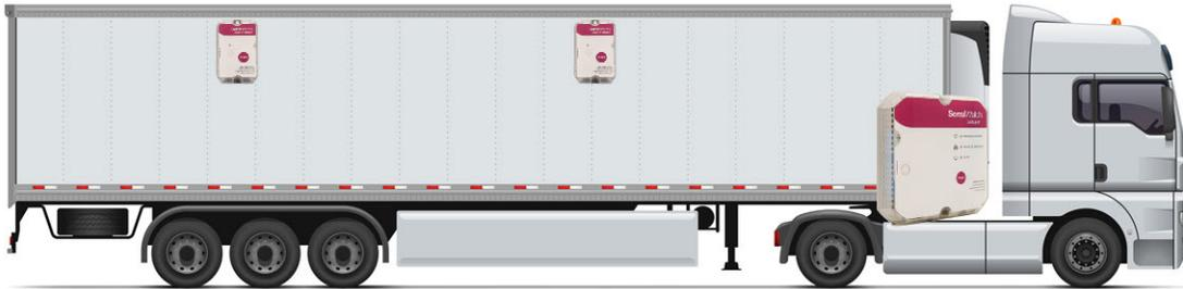
Each Gateway device comes with 2 Remote Sensor devices for refrigerated and frozen zones.
