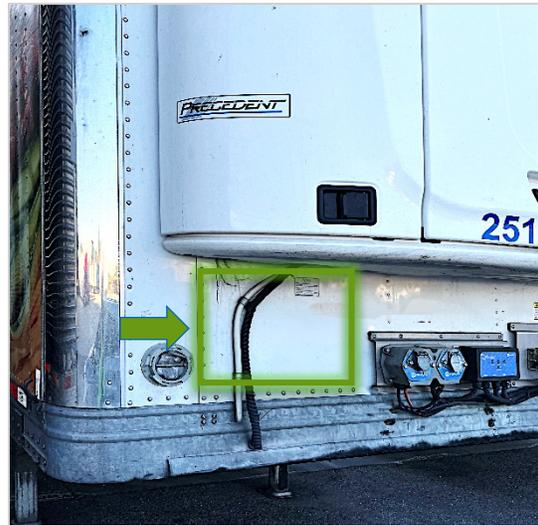
4. Thoroughly clean the surface of the trailer then wipe it dry with a towel to prepare it for the device mounting bracket.
