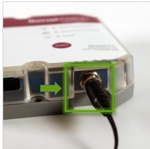
3. Place the Gateway device in the open space on right side, below accessory power outlets.
