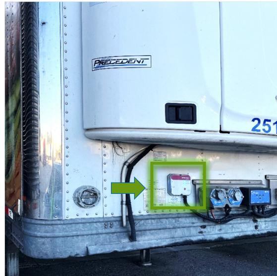
Image of Gateway device attached to lower part of refrigeration unit.
