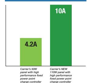
More amps than comparable systems, vital for keeping batteries topped off.
