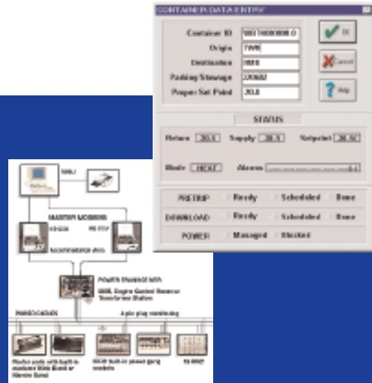
Carrier NT units support three different remote monitoring options. Remote monitoring allows service and operations personnel to monitor the equipment for operating mode and alarm conditions. Some systems support remote pretrip activation, data downloading via the powerline and even remote power saving mode activation. Support for powerline remote monitoring is ISO 10368 compliant.
