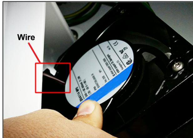
4. Remove the grille and fan assembly. While removing, rotate the fan assembly to in order to expose the wires, see [Figure 7.15](#).
