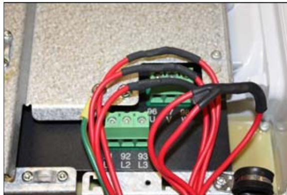
12. Install wire harness clamps and secure the wires using best practice to prevent damage.
