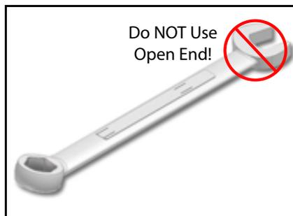
3. Using a deep well socket or box end wrench, turn the transducer assembly counterclockwise to loosen and remove the defective transducer.
