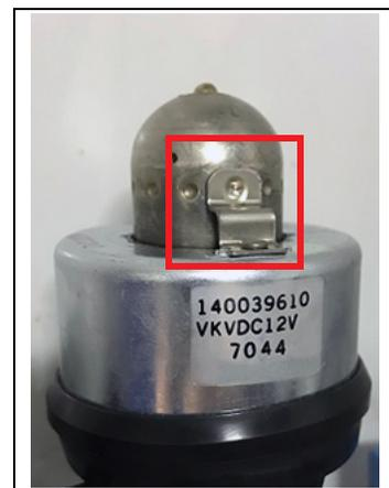
5. Apply the blue dot on the unit side wall next to the coil indicating that the coil has been inspected and is seated correctly on the valve body.
