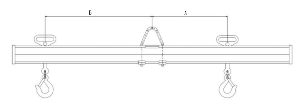
AND: USE 2 LIFTING STRAPS: -1 WITH A HOOK -1 WITHOUT HOOK RESPECTING WEIGHT INDICATED IN CHART
