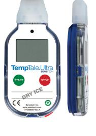
Sample running display Current temperature reading, no alarm
